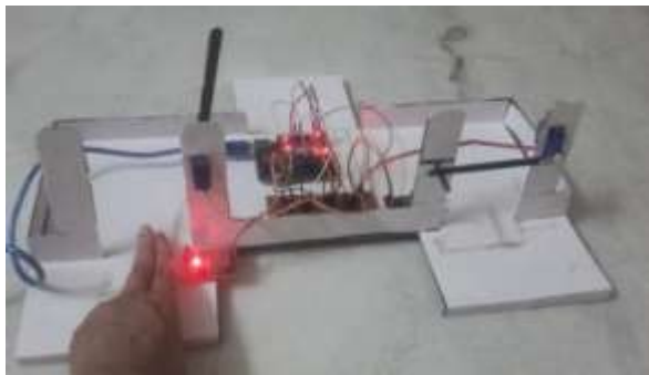
FIG 5: The entry gate sensor detects obstruction shown by glowing of red LED and the gate opens
