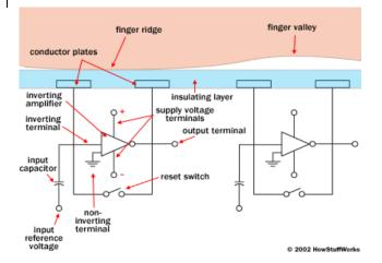
Like optical scanners, capacitive fingerprint scanners generate an image of the ridges and valleys that make up a fingerprint. But instead of sensing the print using light, the capacitors use electrical current.
