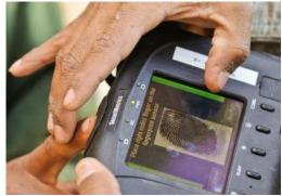
The fingerprint recognition involves snapping an image using a fingerprint scanner which is then digitally compared with a previously stored snapshot of your fingerprints. The scanner processor sees whether the loops, whorls and curves have any similarity. An important point to be noted is that the scanner doesn't keep the complete image of your fingerprint. It only stores information about specific points in the form of binary numbers.
