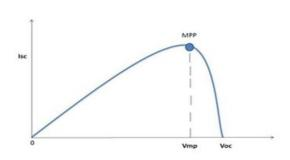
MPPT stands for Maximum Power Point Tracking. MPPT charge controllers used for extracting maximum available power from PV module under certain conditions. According to figure-3 We can see that the maximum power point (MPP) of a solar panel lies at the knee of the current and voltage curve.
