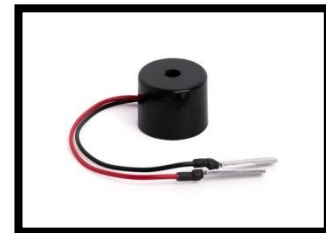
Figure: 5 a buzzer that is used in smart cane as sound Components
