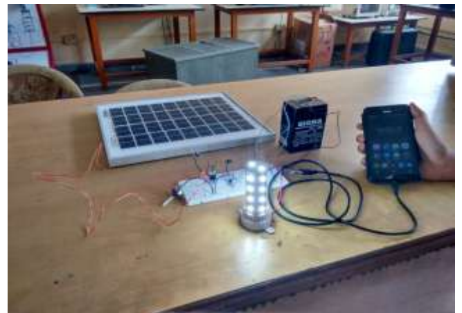
Fig.7. Discharging of batteries with led light
