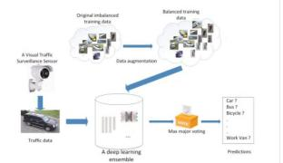
Fig 2. The framework of deep CNN ensemble model [5].
