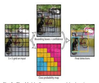
Fig 5: The Model. Our system models detection as a regression problem. It divides the image into an  $S \times S$  grid and for each grid cell predicts B bounding boxes, confidence for those boxes, and C class probabilities. These predictions are encoded as an
