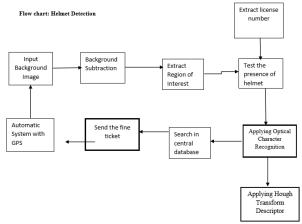
Fig 3. Helmet Detection flow chart [6]
