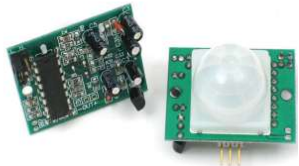
Fig3. Image showing Front and Back side of a PIR Sensor
