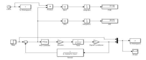
Fig. 4: Model of PID Controller by using MATLAB Simulink.
