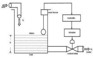
Fig. 3: Schematic diagram of over headed water level control system.
