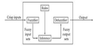
Fig. 2: Basic Configuration of FLC system.
