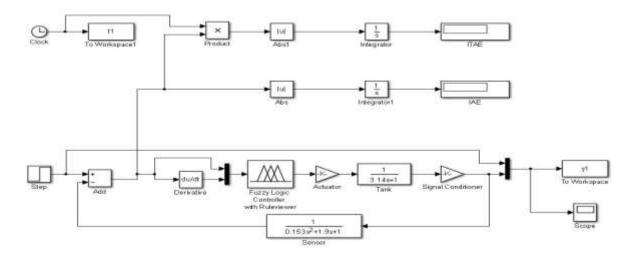
Fig. 6: Model of FLC Block by using MATLAB Simulink.
