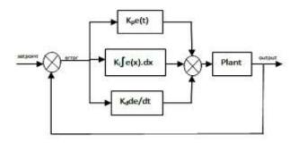
Fig. 1: Block diagram of conventional PID controller.
