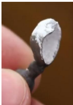
Figure 8. Crown after Casting Process [13]
