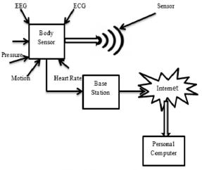
Figure 1: Hardware Architecture
