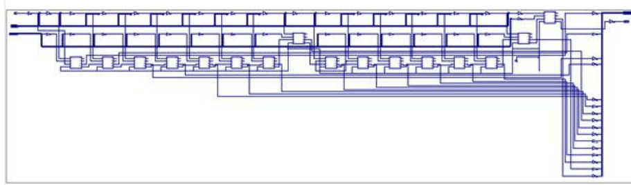
RTL SCHEMATIC OF 16 BIT ADDER USING HNG GATE
