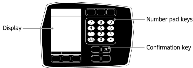
Fig.2: Layout of the mixture pump client interface under study
