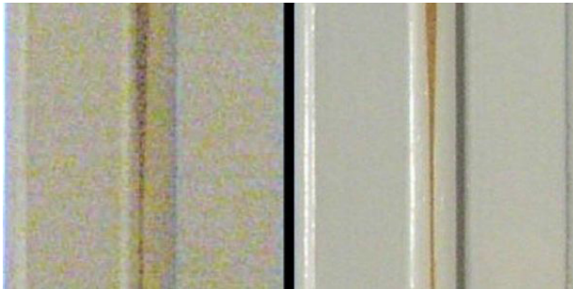
Figure 13: Non- Isotropic Noise with column noise [13].
