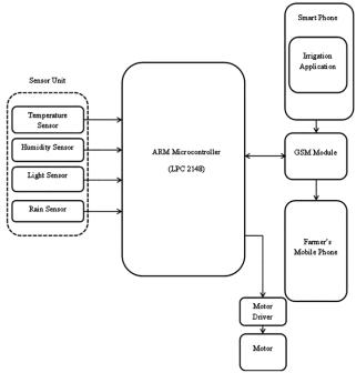
Fig. 3. Block diagram of proposed Smart Sensor based irrigation system.
