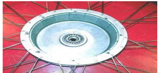
Fig 2: Hub Motor Rotor
