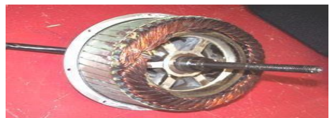
Fig 3: Hub Motor stator
