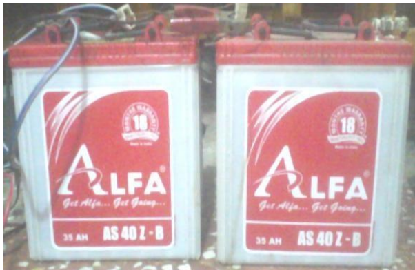
Fig 8: Lead Acid Battery
