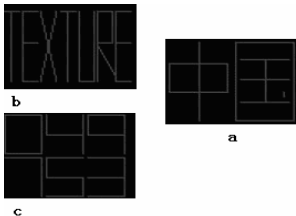
Figure 5. A set of watermarks composed of the Mojette phantoms with meaningful information. (a).a watermark containing two Chinese characters meaning China (b) a watermark which is an English word 'texture' (c) a watermark which is the code of a traffic police office
