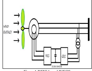
Figure1 DFIG based WECS
