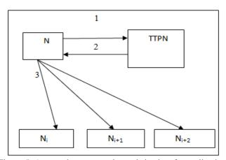
Figure 5: A trusted storage node sends its data for replication to other trusted storage nodes.
