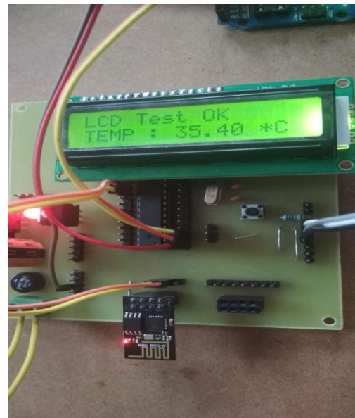
Fig. 4 Test result of Temperature Sensor
