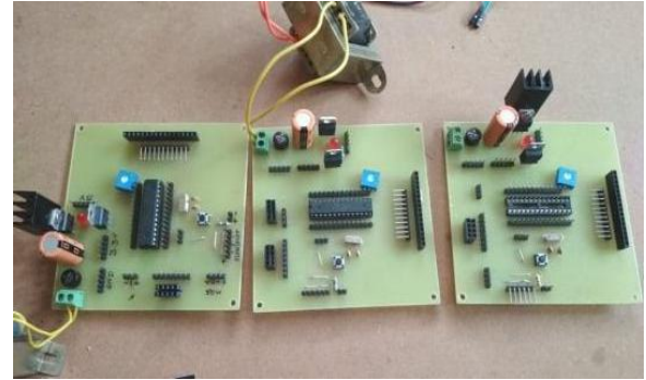
Fig. 3. Gas leak detection PCB designed by schema
