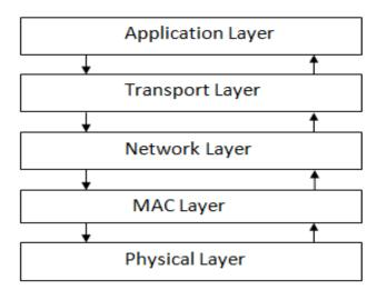
Figure 1. Wireless sensor networks protocol stack.
