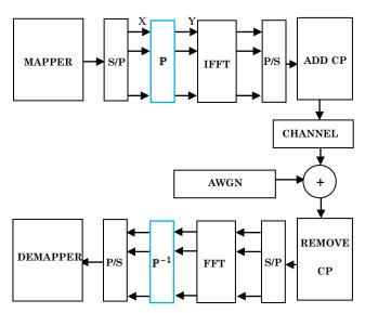
Fig.1 Block diagram of pre-coding based OFDM system
