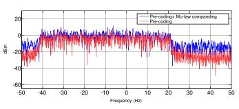
Fig.7 PSD of  $\mu$ -law companded Localized DFTS-OFDM which used zero padding in the end of bit stream (with  $\mu$ =255)
