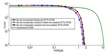
Fig.4 CCDF of various types of OFDM systems
