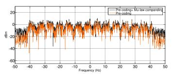
Fig.8 PSD of  $\mu$ -law companded Distributed DFTS-OFDM (with  $\mu$ =255)
