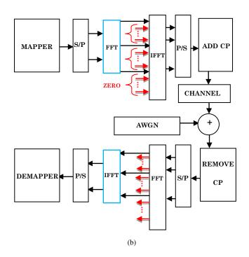
Fig.2 Block diagram of DFTS-OFDM system with (a) zero padding technique and, (b) zero interleaving technique
